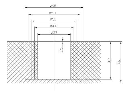
Select the correct diameter compression seal. Remove The smaller seals to match to the larger cable size selected.
