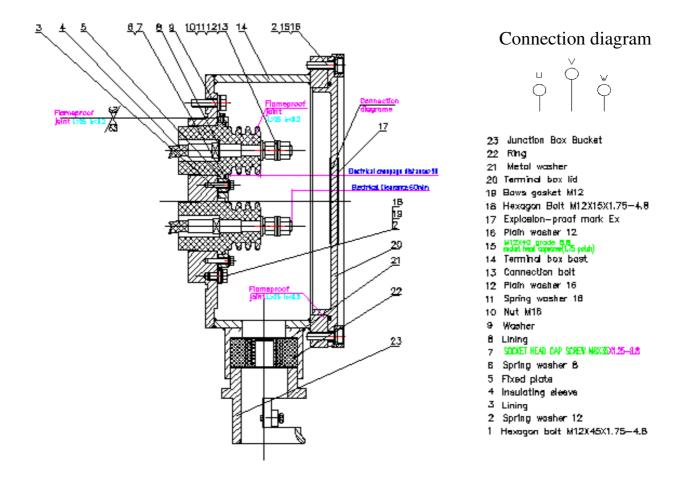
b) The Earth connection. There are Earth connections fitted to the Ex motors, inside the main & aux. terminal boxes, externally on the frame.
