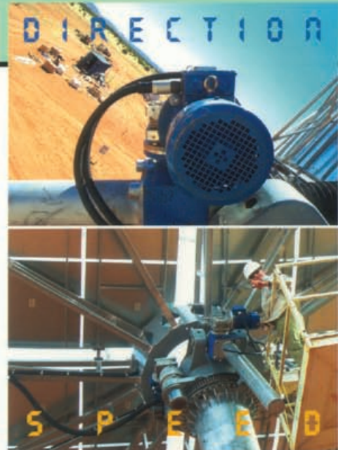
Encoder Tracking on Solar Power Collectors
