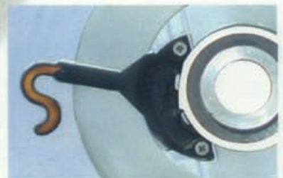
No Contact between Sensor and Rotating Disc
