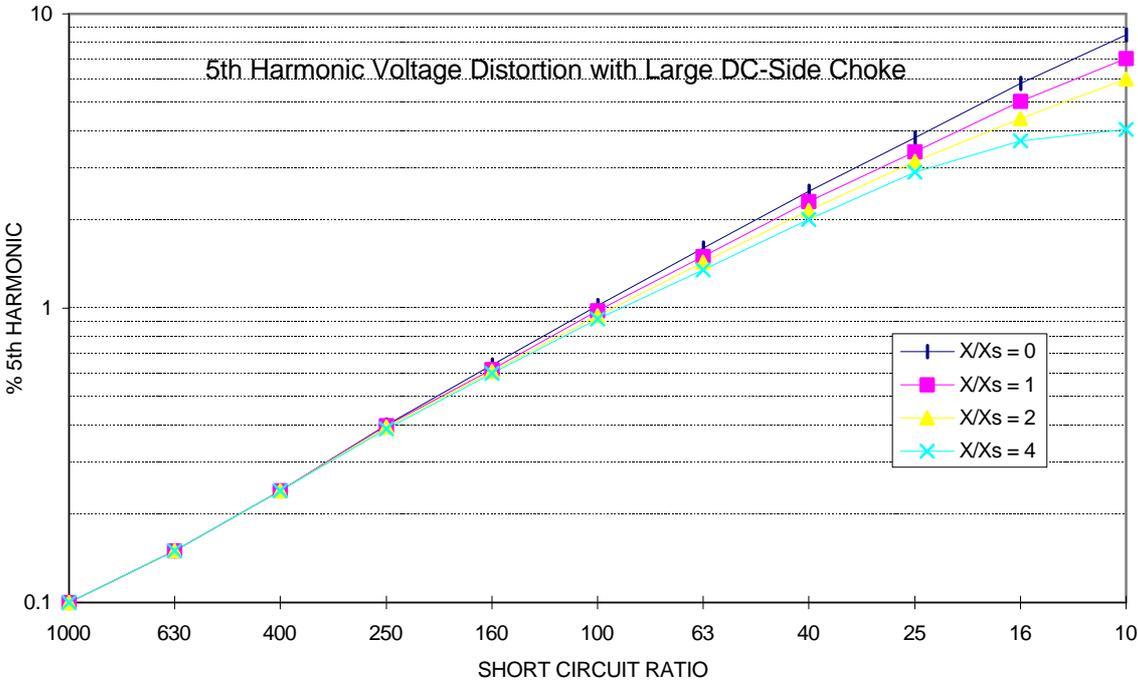
**Figure 2(a):** Percentage of 5th harmonic voltage distortion for a variable speed drive with a large DC-side choke. The effect of AC-side chokes (reactance X) are also shown for various sizes of X. Xs is the supply reactance.
