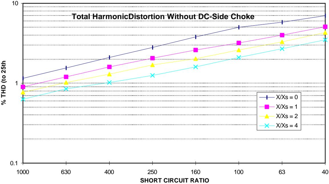
**Figure 2(d):** Percentage of total harmonic voltage distortion for a typical variable speed drive without a DC-side choke. The effect of AC-side chokes (reactance X) are also shown for various sizes of X. Xs is the supply reactance.
