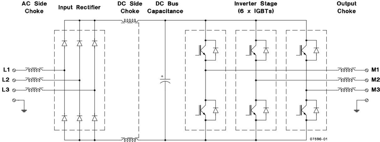
**Figure 1:** Power circuit of a Variable Speed Drive Inverter showing the DC-side choke, DC bus capacitor, input rectifier and inverter output stage and AC-side input and output chokes.
