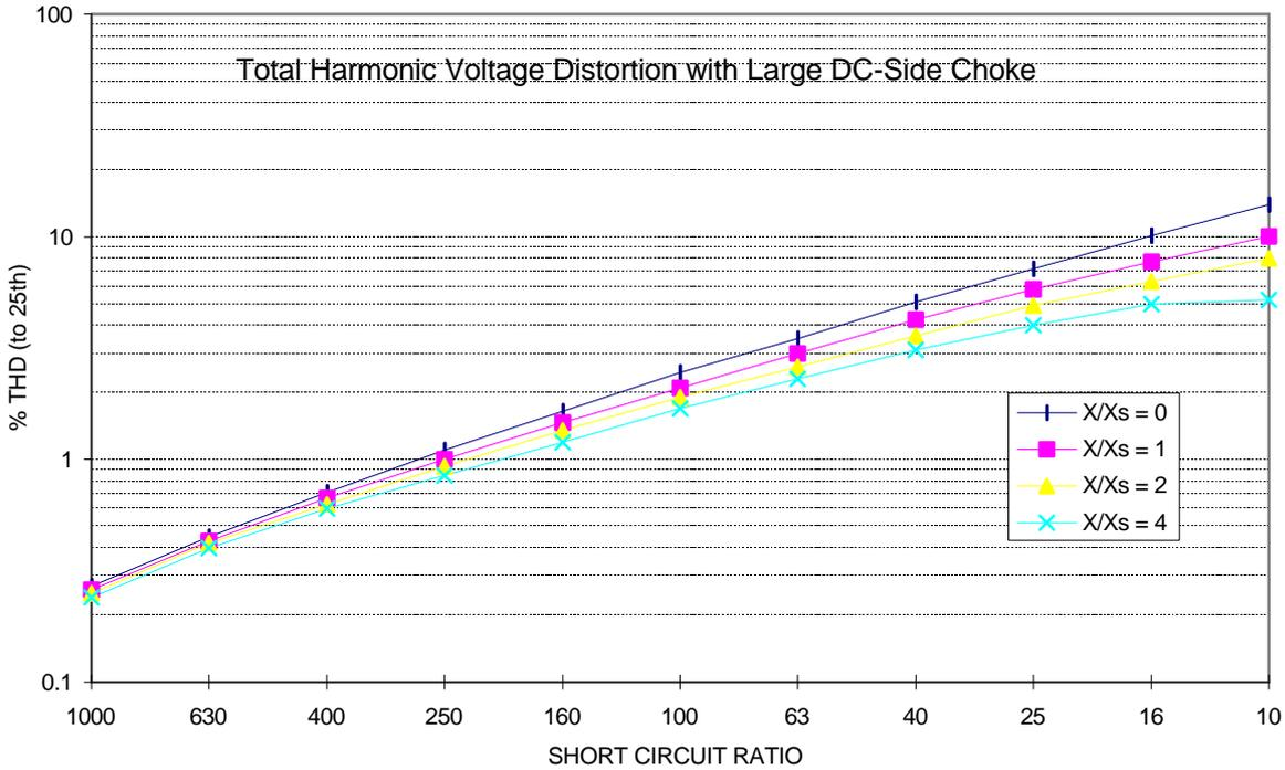
**Figure 2(b):** Percentage of total harmonic voltage distortion for a typical variable speed drive with a large DC-side choke. The effect of AC-side chokes (reactance X) are also shown for various sizes of X. Xs is the supply reactance.
