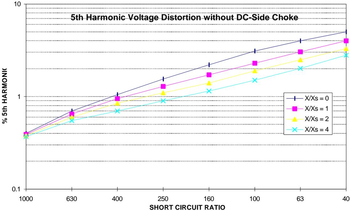
**Figure 2(c):** Percentage of 5 th harmonic voltage distortion for a typical variable speed drive without a DC-side choke. The effect of AC-side chokes (reactance X) are also shown for various sizes of X. Xs is the supply reactance.
